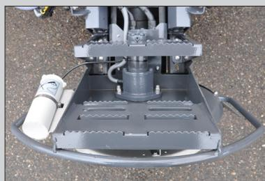
Wide steps on the spreading disc arrangement means safe and easy access to the engine compartment.
